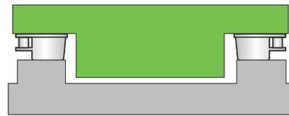
Vibration insulation concrete block or steel platform
